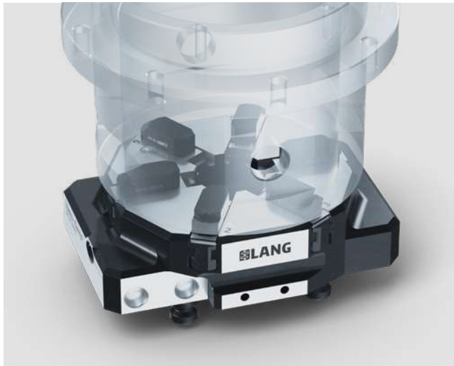
Vasto-Clamp with 6 hardened gripping jaws for I.D. clamping.
